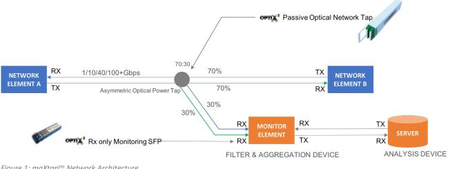
Figure 1: maXtap<sup>tm</sup> Network Architecture
